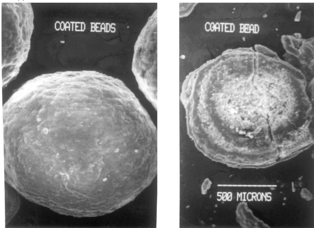
Fig. 9. SEM pictures of coated beads and its cross-section.
